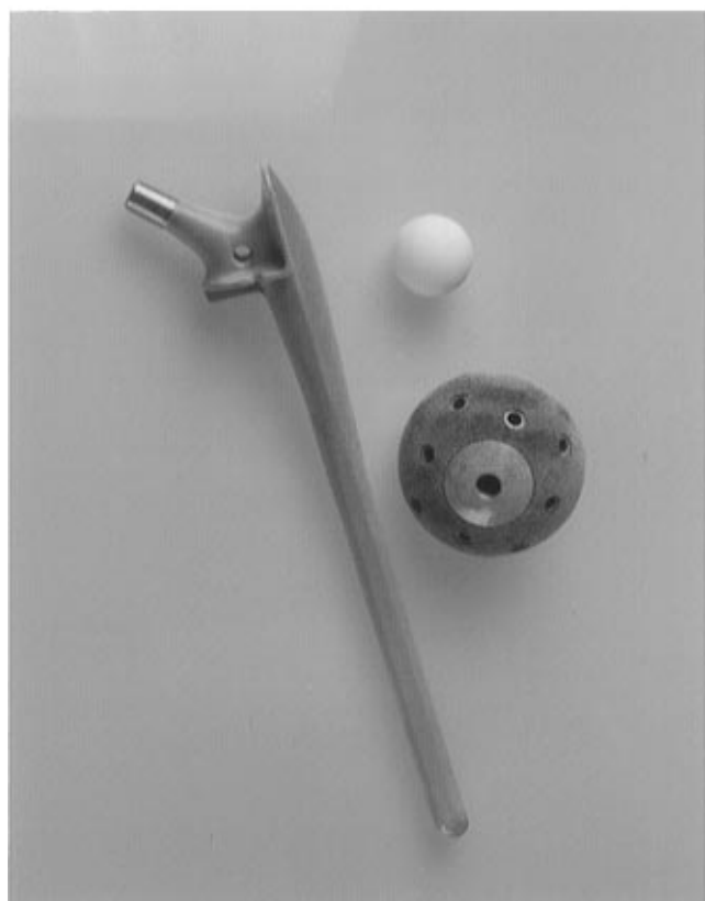
Figure 4. Titanium hip implant coated with a thin, coherent hydroxyapatite layer.
